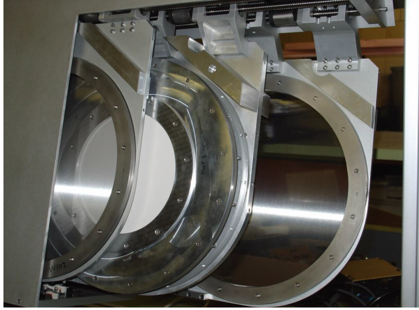
Figure 2.5: The three blades that combine to form POL-2 are partially extended showing the two wire grids and the achromatic HWP. The two wire grids are the calibrator grid and the analyser grid. The rotating HWP is located between these two fixed grids. The calibrator grid is only inserted for test purposes. Stiffeners can be seen on all three blades. The one for the HWP is particularly thick. Their purpose is to reduce vibrations while the HWP spins.
