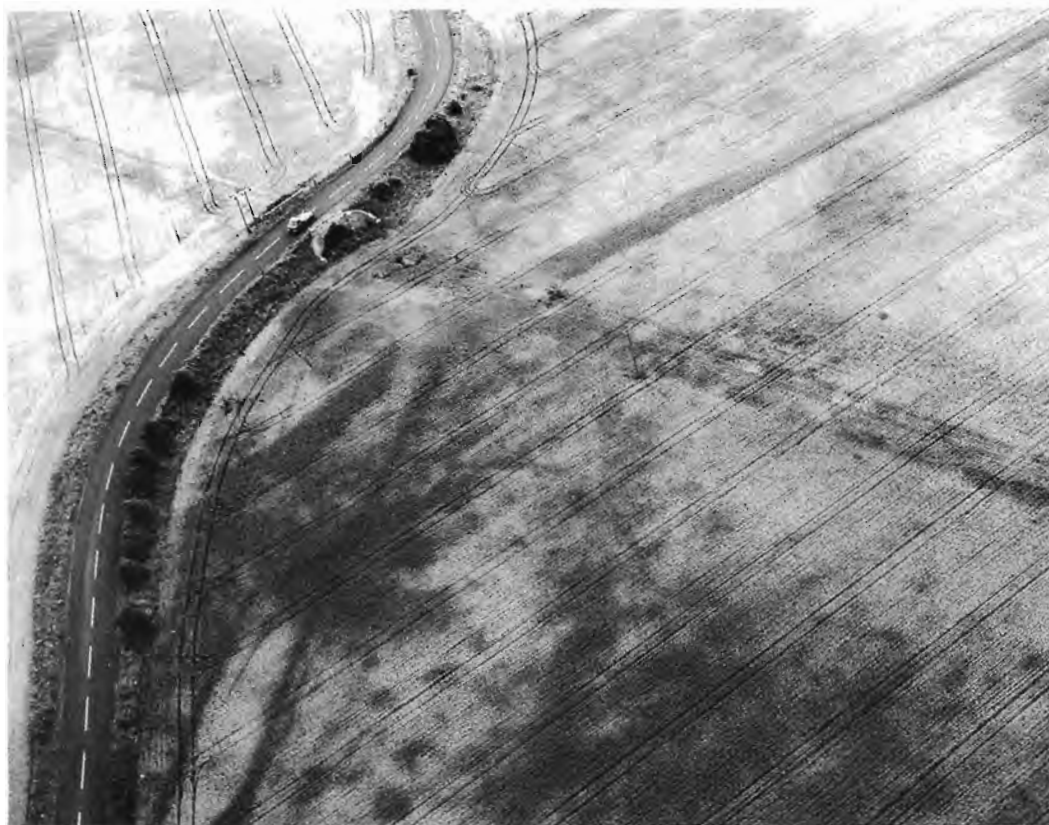
Illus 4.28. The S-bend at Waterless Bridge which carries the road across the demolished 1865 railway, visible as a crop mark running diagonally across the picture. Parallel crop marks to the right of the present road may be identified as the side ditches of its pre-railway predecessor.
