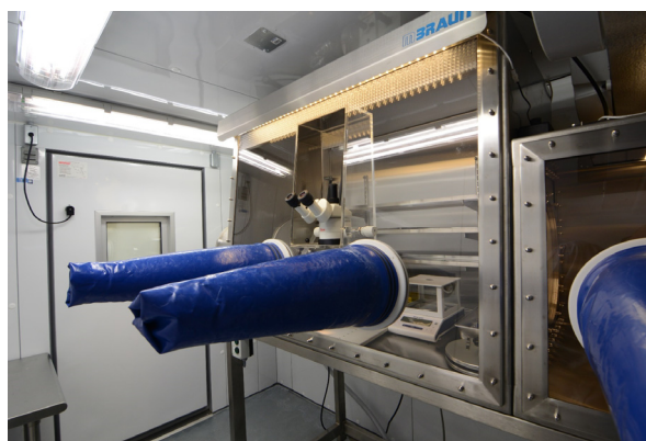
Figure 1. Ar glove box within freezer, after [4].
