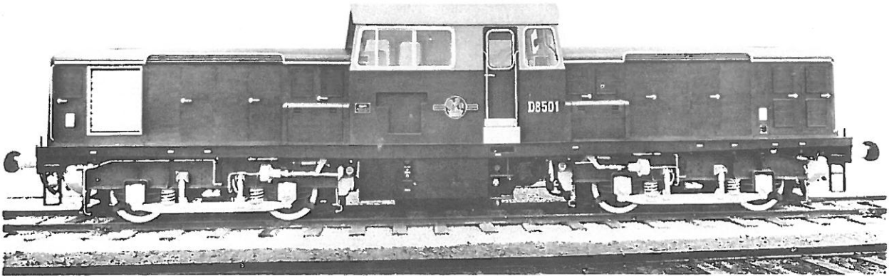
Fig. 1—New type 1 locomotive showing the centre cab with a 450 b.h.p. power-unit mounted over each bogie
