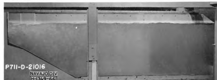
Discharge = 3,625 cfs T. W. El. 5718
