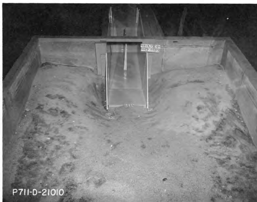
C. Erosion after one hour model operation
