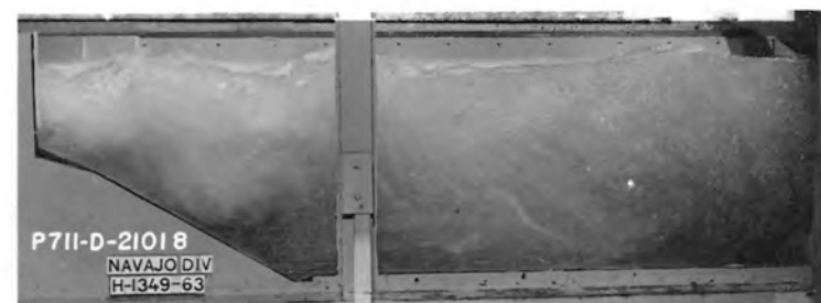
Discharge = 10,875 cfs T. W. El. 5722
