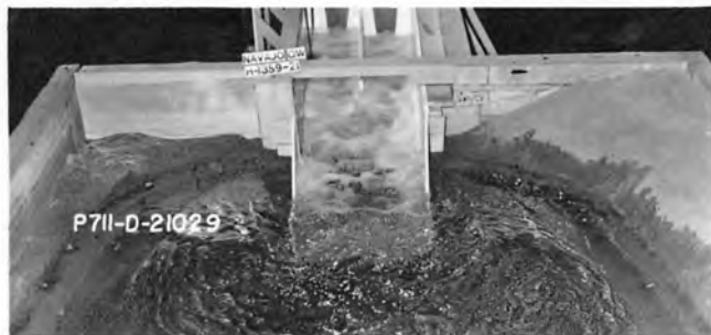
A. Valves 50% open, Head 166 feet, T.W. El 5711
