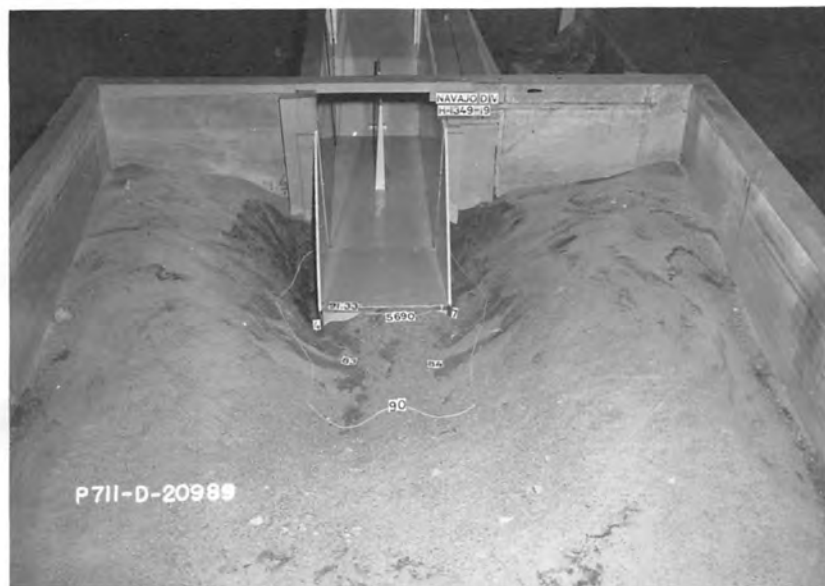
B. After one hour model erosion test 14,500 CFS - Tailwater elevation 5718.5
