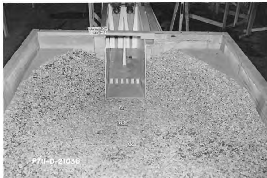
B. Head at valves 100 percent open 217 feet. Tailwater elevation 5713. Erosion pattern in riprap after 5 hour model test run.
