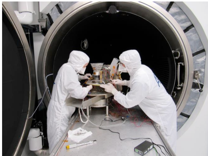
Engineers at the Johns Hopkins Applied Physics Laboratory prepare one of Europa Clipper's cameras for testing. Credit: NASA/APL/Ed Whitman
