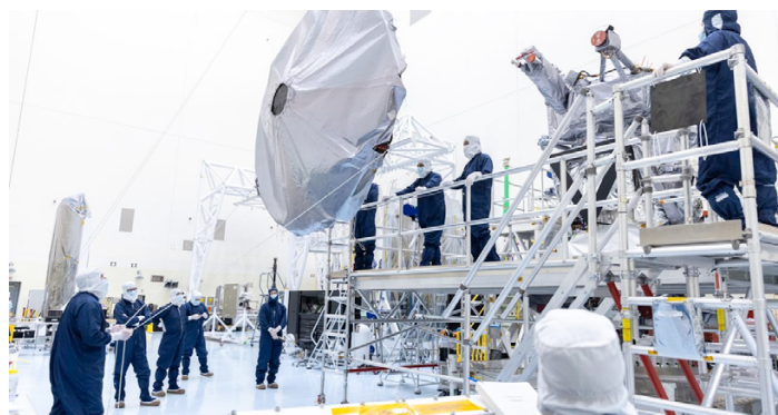
Technicians at NASA's Kennedy Space Center prepare to install Europa Clipper's 10-foot (3-meter) high-gain antenna. Credit: NASA/Kim Shiflett
