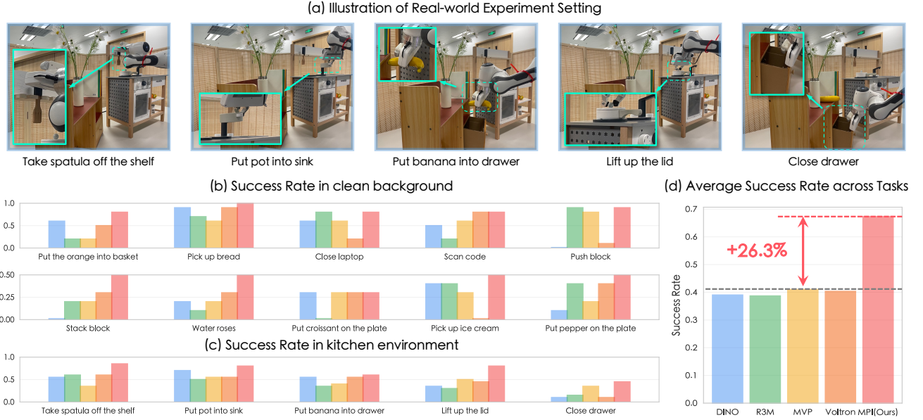
Fig. 3: Real-world robot experiments. (a) Illustrations of real-world experiments in the kitchen environment. (b) Detailed success rate of ten tasks within a clean background. (c) Results of five tasks in the complex kitchen environment. (d) MPI outperforms previous state-of-the-art with an average elevation of 26.3% success rate across 15 tasks.
