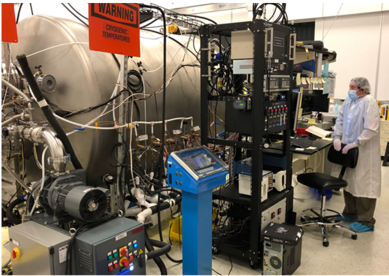
Fig. 20 The Thermal Vacuum Test Facility in ASU's School of Earth and Space Exploration that was used for E-THEMIS TVAC testing
