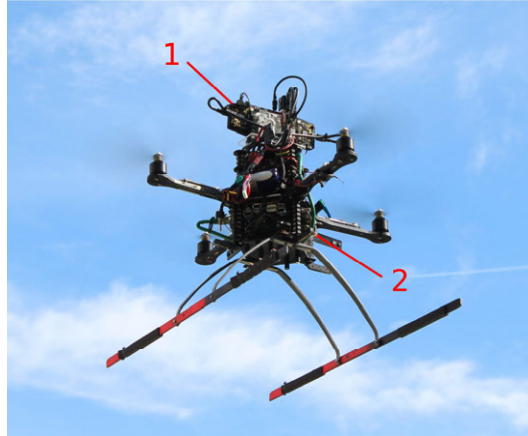
(b) Quadrotor UAV field test. 1) stereo vision system. 2) onboard host computer.
