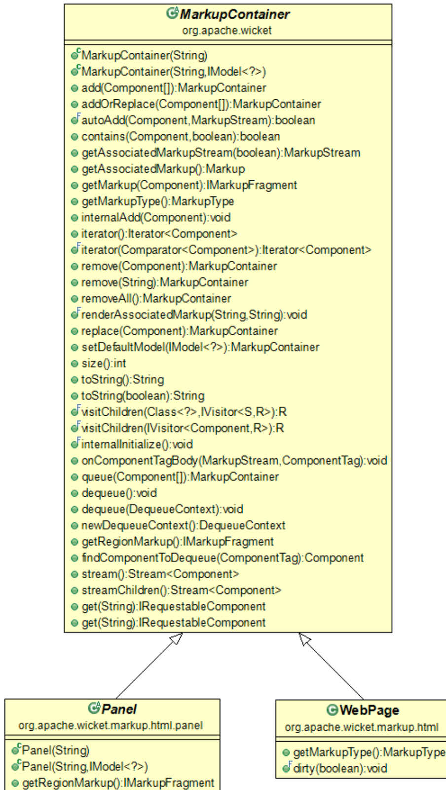
Illustration: Hierarchy of WebPage and Panel classes
