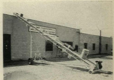
PORTABLE CONVEYOR can carry variety of materials up a fairly steep slope to a roof.
