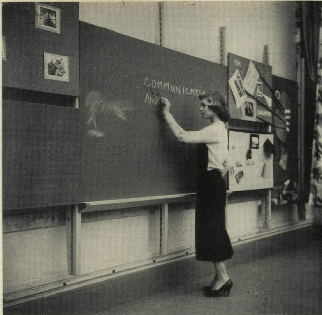
Flexible wall has permanent standards, metal holders for interchangeable boards, shelves, racks. Stock system is adapted from Ketchum, Gina & Sharp custom design (AF, Dec. '54).
