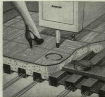
Sketch of Cellufloor installation in Federal Reserve Bank Building
